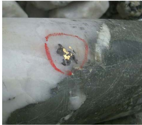
Above: Drill core showing Gold surrounded by Sphalerite a Zinc mineral which is often associated with nuggety gold.
